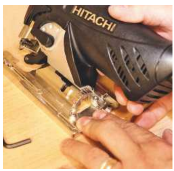
▲ Base adjustment is with a hex key, sliding the base forward to set angles
